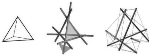
Fig. 3 Polyhedron, Polyhedral Weave-Sticks and Polyhedral Tensegrity [7]
