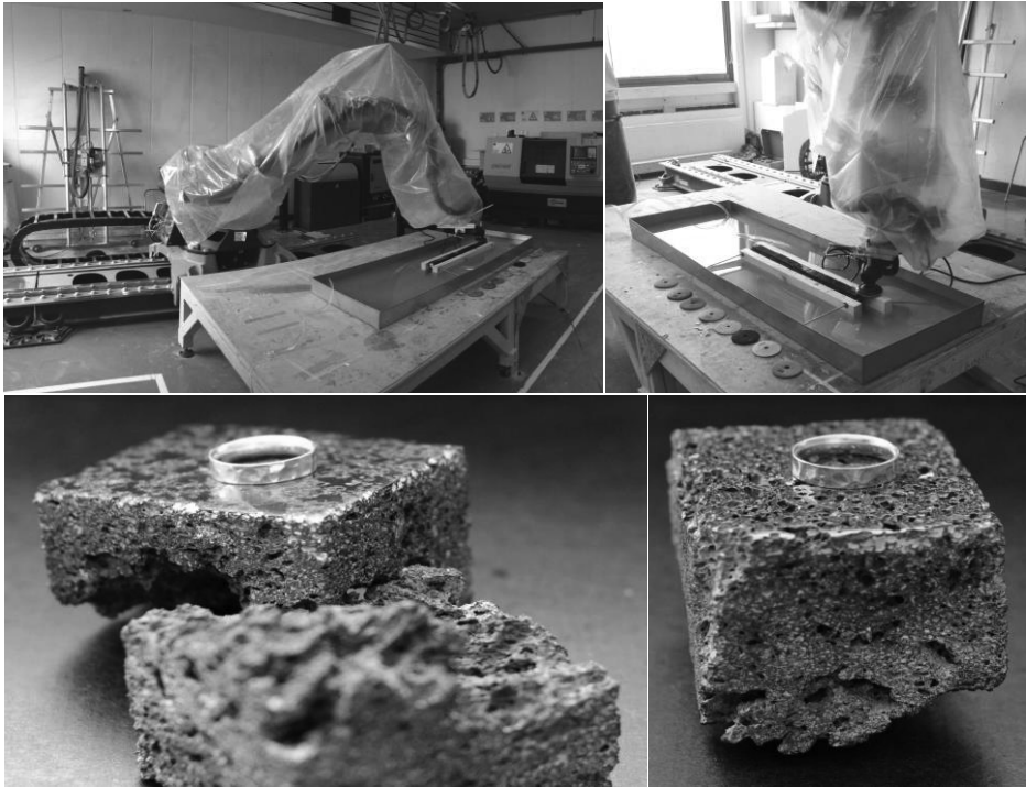
Fig. 9. Polishing setup. / First polishing results
