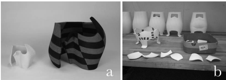
Fig. 5. Prior study, the decomposition of an initial shape using straight cuts. Current study using spline curves to decompose the initial shape.
