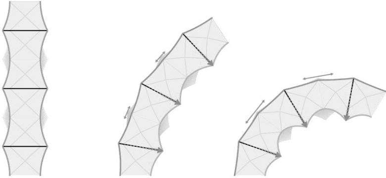
Fig. 18. Damping system for tensile skin using bars
