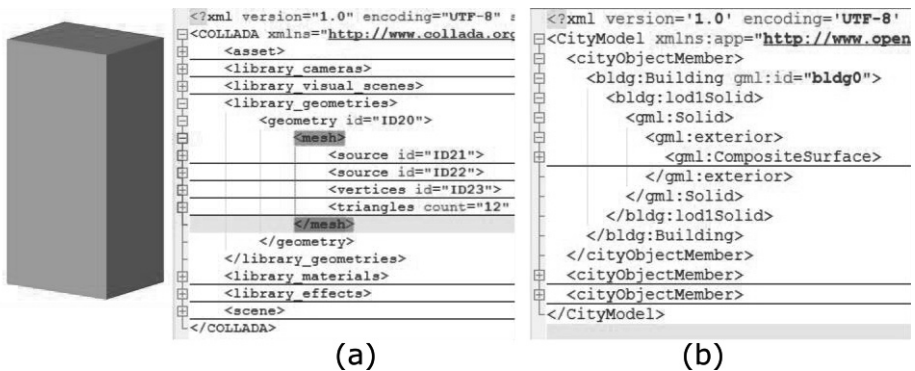
Fig. 5. (a) Building extrusion exported as Collada from SketchUp (b) Converted CityGML building extrusion with explicit building semantic information.
