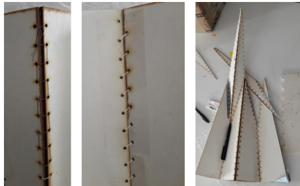
Fig. 20. Plywood stitching (Source: Authors)
