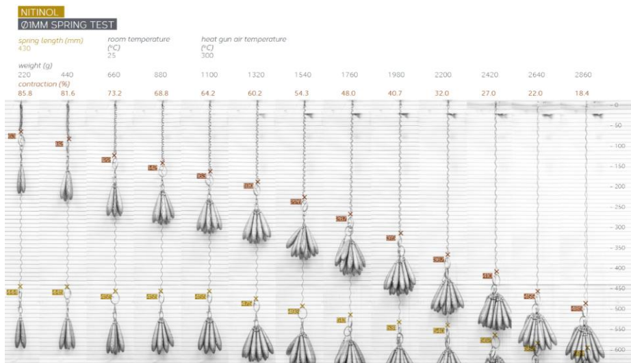
Fig. 3. Nitinol springs strength test
