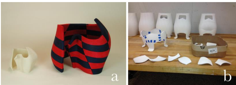
Fig. 5. Prior study, the decomposition of an initial shape using straight cuts. Current study using spline curves to decompose the initial shape.
