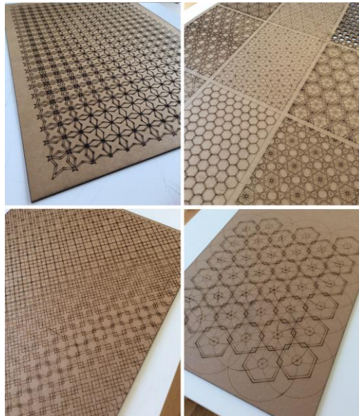
Fig. 7. The models with different geometries, which were made by using cardboard material and produced by doing laser scoring
