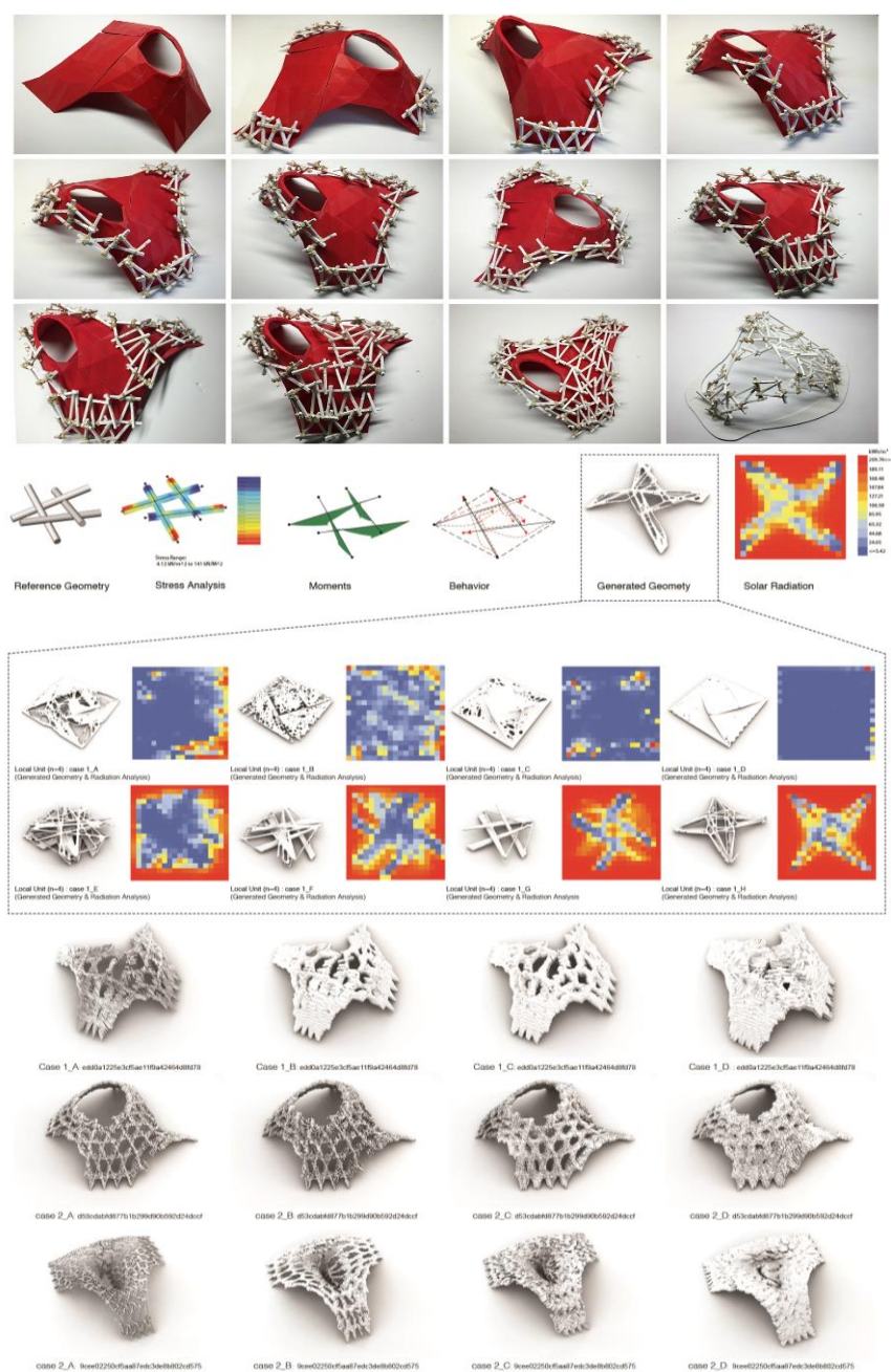
Fig. 9. An illustration of design exploring the erection sequence study performed manually (top); a set of simulated frames illustrating the cementitious deposition and resultant shading analysis (middle); and a set of 3 global configurations illustrating a variety of agent driven porosities (bottom).
