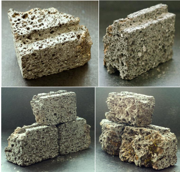
Fig. 8. Peg and socket joints first roughing test. Front / Back views.
