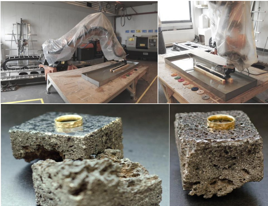
Fig. 9. Polishing setup. / First polishing results.
