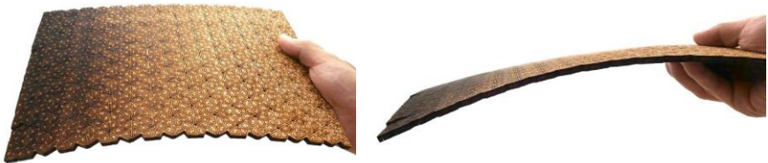
2. When the pattern in Fig.1a is used for kerfing a planar wood panel, it turns a rigid wood panel into a gradually flexible rectangular panel which is rigid in one side and flexible in another.
