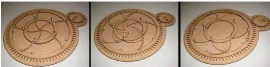
Fig. 8. Mechanical Iris mechanism, final structure and motion (Project B)
