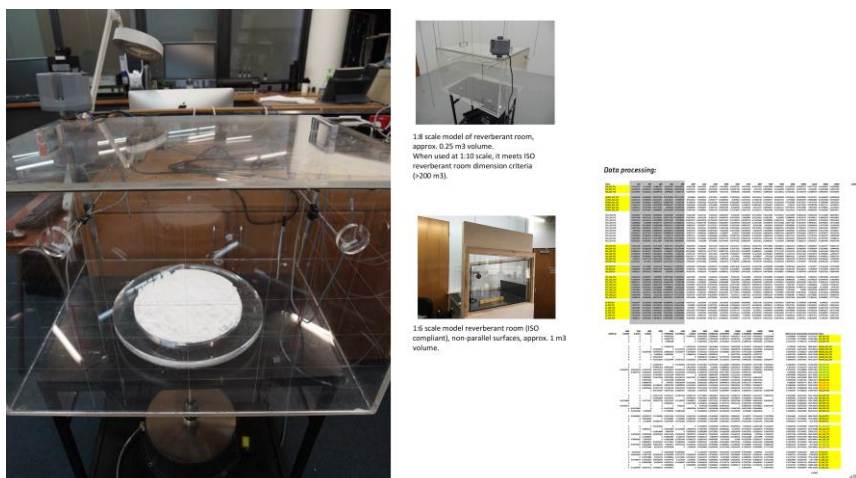
Fig. 4. Scale model reverberant room (right, mid) and scattering data (left) from scale model prototypes.
