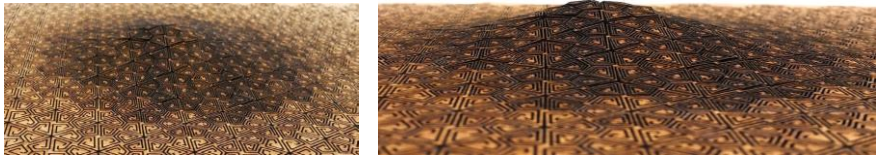
(b) When the pattern in Fig. 2a is used for kerfing a planar wood panel (also called relief cut), it makes the center of the wood panel flexible by allowing to turn it into a conical dome structure.
