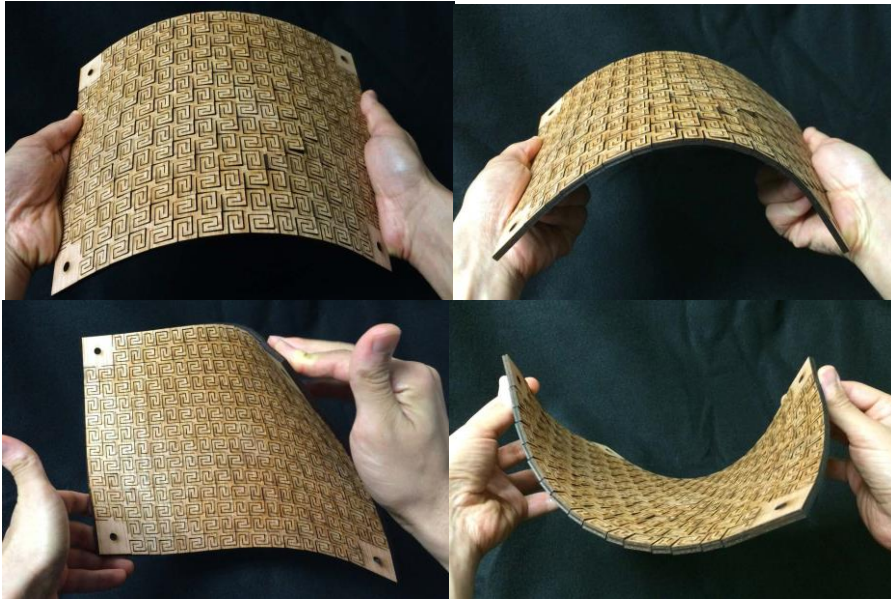
(c) We created these models using our generalized algorithm to demonstrate that our algorithm can produce the original 2D-meander-pattern and its flexibility.
