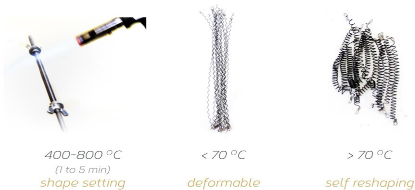
Fig. 2. Nitinol – shaped into springs, stretched and reshaped by heat
